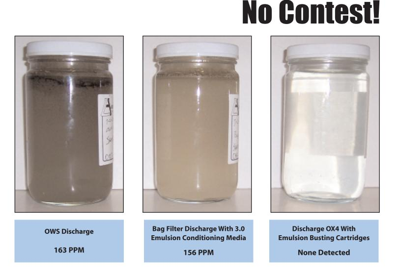
The above samples were taken from a 6 month old OWS onboard an oil tanker that has emulsified oil problems. The first sample was taken from the OWS without any of our OIL-XORB filters installed. The second sample was taken with our Bag Filter installed to condition the oil being sent to the emulsion busting cartiridge filters. The final sample is the discharge from our OIL-XORB cartridge filter using the emulsion busting blend.
