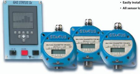
The Gas Status Sx is designed as a cost effective and reliable fixed sensor solution for continuously monitoring gas concentrations in the pump room. Intrinsically safe INFRA-RED combustible sensors can be located in up to 6 locations within the pump room. Additionally, an oxygen sensor and/or a hydrogen sulfide sensor can be connected to the system.
